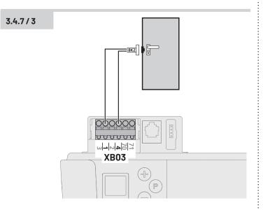
After connecting the accessory and the subsequent mains On, the controller automatically detects the accessory.
