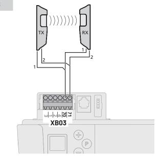
A connected photocell is automatically detected by the controller as soon as the power supply is connected. The photocell can be retrospectively reprogrammed.
