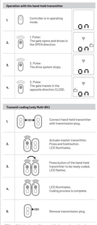
With multi-button transmitters, each button can be assigned a separate function.
